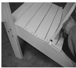
Place Back Assembly on top of mounting surface of Rear Legs, (Left Picture). Push Back Assembly forward until it's aligned with Seat Assembly. Hold Back Assembly in place and install (4) Robertson Head Screws into the base on each side. There are no predrilled holes, you need to align the horizontal bar with the sides of the base, making sure that the base of the backrest aligns with the seating surface.
