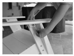
Arms should be installed with curve side on the outside of the chair. (Left Picture). Place Arm on top of Front Leg. Align pre-drilled hole in arm with the pre-drilled hole located at the top of the Front Leg. Install a short connector bolt through pre-drilled hole in the Front Leg, then through pre-drilled hole under arm. Install flat washer, lock washer and nuts. Do not tighten at this time. Repeat process on other side.
