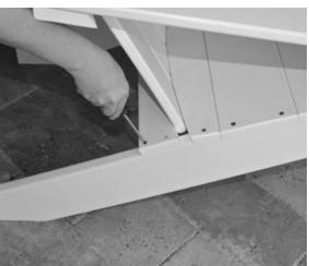
Place Back Assembly on top of mounting surface of Rear Legs, (Left Picture). Push Back Assembly forward until it's aligned with Seat Assembly. Hold Back Assembly in place and install (4) Robertson Head Screws into pre-drilled holes on each side. There are no predrilled holes, you need to align the horizontal bar with the sides of the base, making sure that the base of the backrest aligns with the seating surface.
