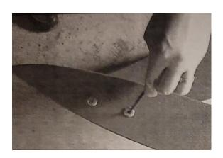
Attach the runners to the front using (2) 1-1/4" wafer head bolts and to the back using (2) 2-3/4 "wafer head bolts.
