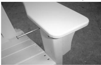
Arms should be installed with curve side on the inside of the chair. (Left Picture). Place Arm on top of Front Leg. Align pre-drilled hole in arm with the pre-drilled hole located at the top of the Front Leg. Install a short connector bolt through pre-drilled hole in the Front Leg, then through pre-drilled hole under arm. Install flat washer, lock washer and nuts. Do not tighten at this time. Repeat process on other side.
