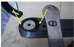
The bobbin case holder must be positioned as shown in the photo. The holder should be directly opposite the needle hole. If the bobbin case holder is not correctly positioned, you can remove it with an awl or other pointed object through the hole in the bottom and then put it back correctly.
