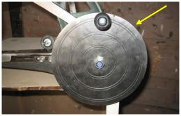
Turn the flywheel handle upwards. The foot should be up. Rotate the bobbin cover/needle plate perpendicular to the lower arm.
