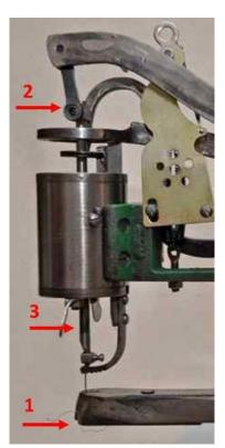
Place the needle, by turning the flywheel, to its lowest possible point. Use your finger to check if you can feel the needle in the needle hole at the bottom of the lower arm (number 1). You should feel the needle just a a little bit.
