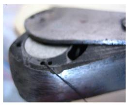
Put the bobbin case back in the machine. Pull the thread at least 10 mm out of the bobbin and place it in the notch. Close the bobbin cover/needle plate.
