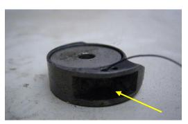
Place the bobbin back in the bobbin case. Pull the thread to see if the bobbin can rotate freely. On one of the bobbin cases there is a copper tab (see arrow). By leading the thread behind this tab the lower thread will be held tighter while sewing. You can change the tension by loosening or tightening the screw.
