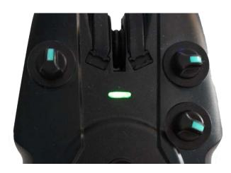
While in the configuration menu the Tone knob adjusts the colour of the Nightlight LED. There are 4 selectable colours: Blue - Yellow - Green - Bed - Off.
