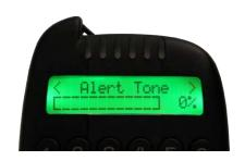
In 'Advanced Menu' go 'Alert Tone' to adjust the pitch on the Alarm and the HUBB.
