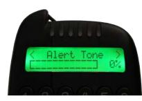
In 'Advanced Menu' go 'Alert Tone' to adjust the pitch on the Alarm and the HUBB.
