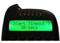
Go to 'Alert Timeout' to adjust the time that the LED remains turned on after an alert on the bite Alarm. 60 seconds / 30 seconds / 20 seconds / 10 seconds /
