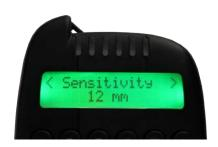
8 Sensitivity Levels, expandable to 16 via HUBB Link 2mm, 6mm, 12mm, 18mm, 25mm,
