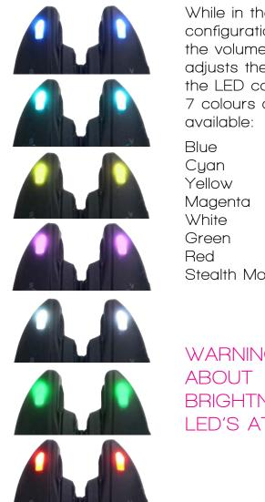
While in the configuration menu the volume knob adjusts the colour of the LED colours. 7 colours are
