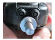
When IQ Port or Smart LED Port are not being used the rubber socket holders should be pressed into ports. When not needed they should be pressed into the socket holders on reverse of Alarm.
