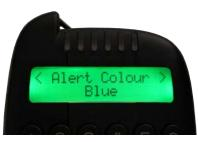
Go to **'Alert Colour'** to change the colour used to display alerts on the bite Alarm and HUBB.
