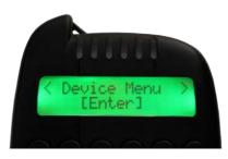
on the HUBB and the HUBB LED's should replicate the alert colour shown on the bite Alarm. Depending on the HUBB's settings, the HUBB will also vibrate on alert. When **'Device Menu'** is shown, use OK button to enter sub menu.
