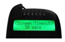
Adjust the time of inactivity before the screen turns off.
