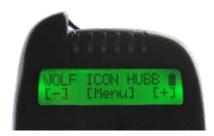
From the main screen, press OK button to enter the HUBB main menu. Press • or • to browse through the menu, and use OK button to enter the various options. For most options, press OK button to edit, use • and • to adjust the value, and then OK button to confirm the new value, or • to cancel.
