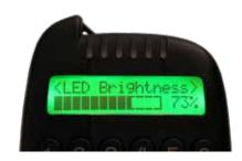
Go to 'LED Brightness' to change the brightness of the LED's displayed on the bite Alarm.
