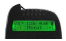
From the channel info screen, press and hold the corresponding channel key to enter the channel menu.
