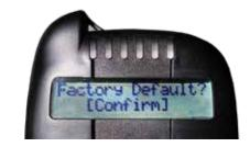
To return the HUBB to factory settings, and clear all user data. power the HUBB off, and then power it back on while holding the (3) key, keep holding the key until the following is displayed.
