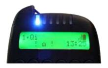
From the channel info screen, press and hold the corresponding channel key for 5 seconds to enter the unpair screen.
