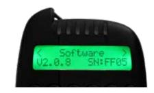
Displays the current version of software and the Serial Number of the HUBB.
