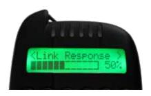
Adjusts the responsiveness of all paired link devices. Electronic system to detect when the devices are still linked, used to ensure you are within the suitable distance from the devices. This is done Manually.
