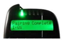
If pairing was successful this will be displayed. Press OK button to confirm the pairing.
