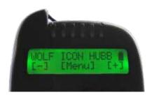
On the HUBB main screen. the HUBB's battery level is displayed. Press and hold the OK button to display the current time and date.
