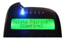
Press OK button to confirm the deletion of this device from this channel.
