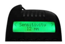
8 Sensitivity Levels, expandable to 16 via HUBB Link 2mm, 6mm, 12mm, 18mm, 25mm, 35mm, 60mm or 100mm. Additional Sensitivity Levels 4mm, 8mm, 16mm, 20mm, 30mm, 40mm, 80mm or 300mm.
