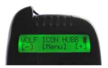
From most screens, pressing a channel key will display the relevant channels paired device info. If channel shown is unpaired. Press and hold 3 for 5 seconds to enter pairing mode.
