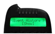
Screen displays a list of recent events from all paired channels. Using the OK button to enter this sub menu the displays recent events in a chronological order. Using the left and right buttons you can navigate through previous events.
